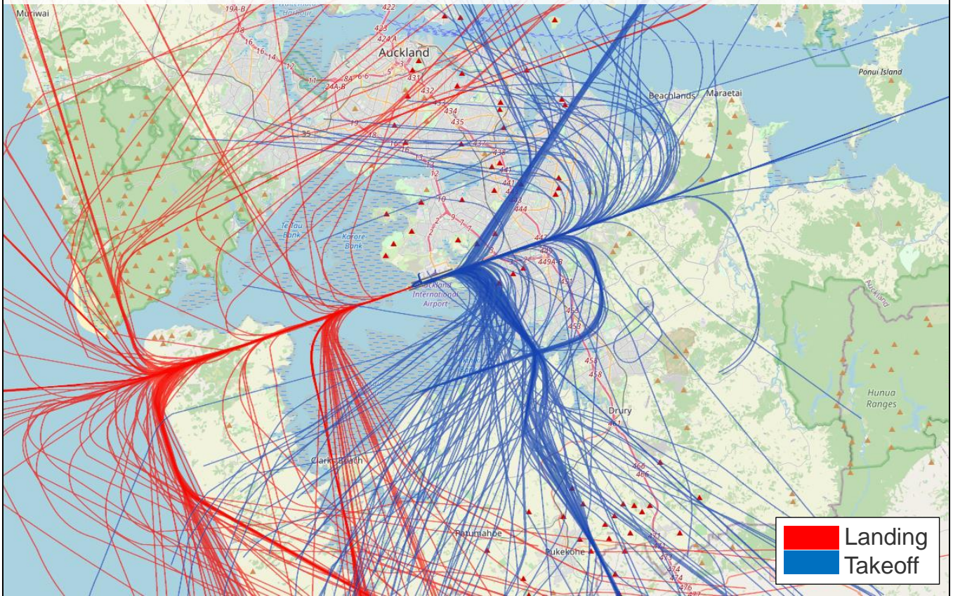
Figure 9: Flight Paths for a Busy Runway 05R Day (7am-10pm) 100% Easterly Winds/Runway 05R
