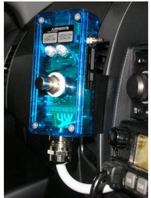
Example Transponder Control Box
